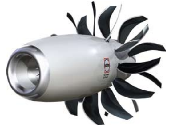
CFM International's open-rotor concept engine
